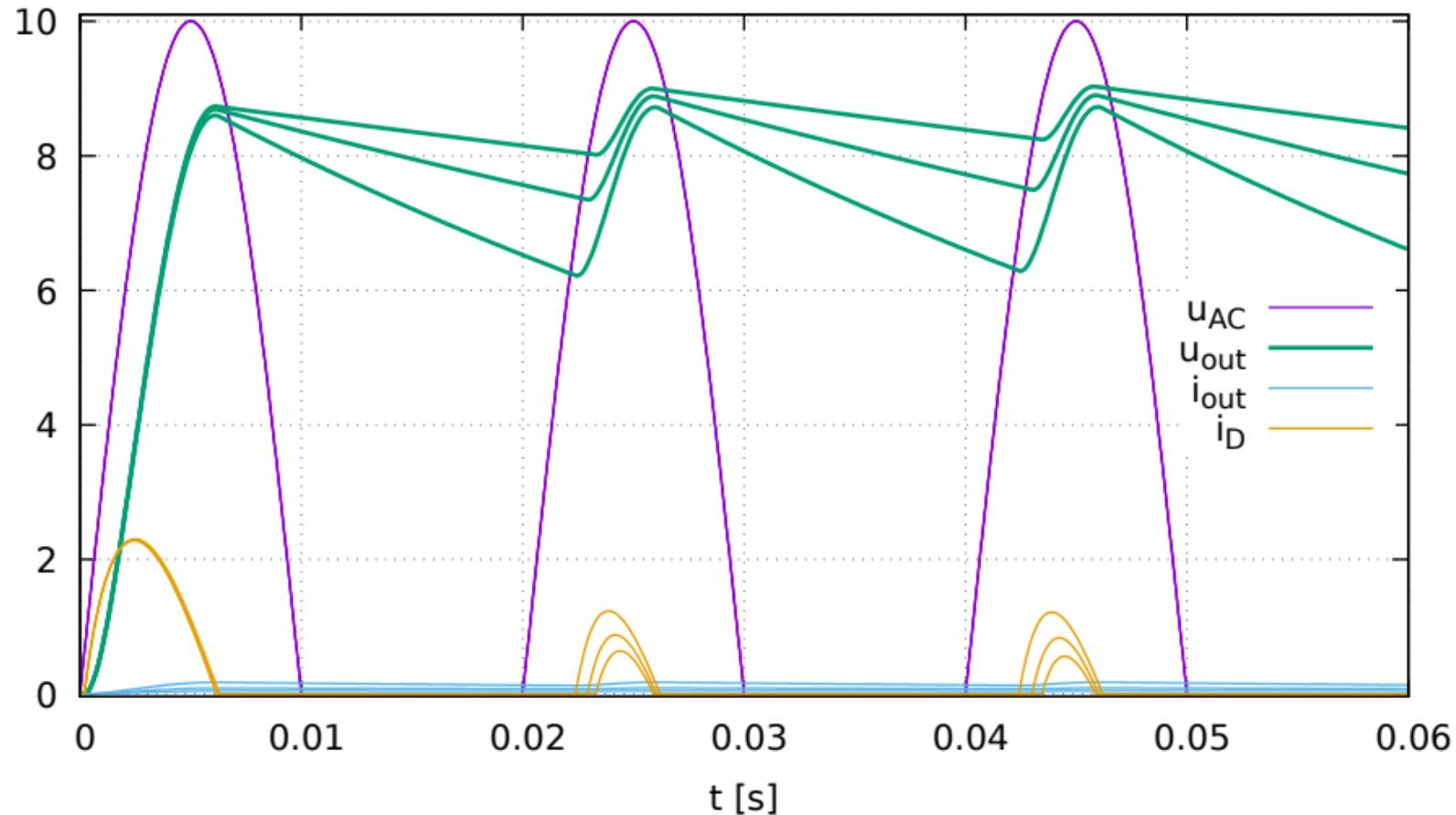
Rectifier ( $U_{AC}=10V/50Hz$ ,  $R_{AC}=1\Omega$ ,  $C=1000\mu F$ ,  $R_z = 50, 100, 200 \Omega$ )
