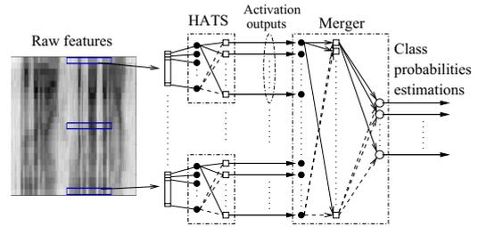
Figure 3: Scheme of HATS architecture.
