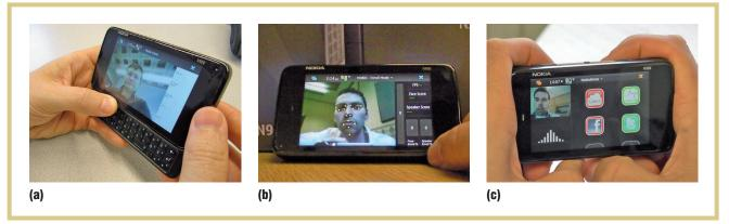
Figure 6. Mobile Biometrics interface demonstrating (a) face detection, (b) facial feature localization (for shape normalization), and (c) the user interface with automated login and logout for popular websites such as email and social networking.
