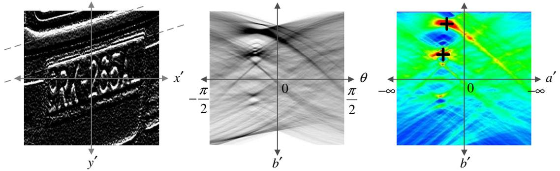
**Figure 2.12:** (a) Number plate in the unified “XY” coordinate system after application of the horizontal edge detection filter (b) Hough transform of the number plate in the “ $\theta B$ ” coordinate system (c) Colored Hough transform in the “AB” coordinate system.
