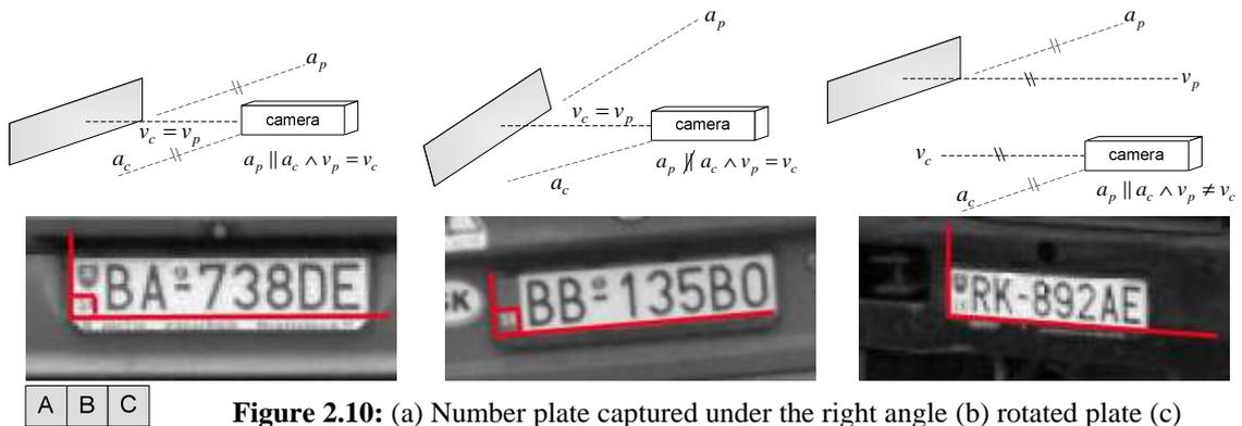
**Figure 2.10:** (a) Number plate captured under the right angle (b) rotated plate (c) Sheared plate
