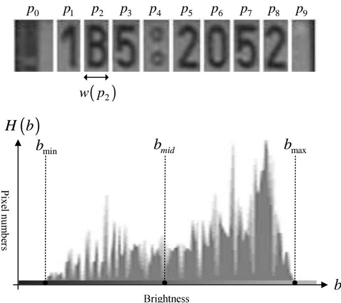
**Figure 2.9:** (a) The number plate must be segmented into individual characters for deeper heuristic analysis. (b) Brightness histogram of the number plate is used to determine the positivity of the number plate.
