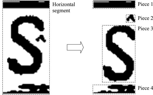
**Figure 3.2:** Horizontal segment of the number plate contains several groups (pieces) of neighboring pixels.
