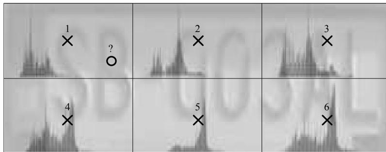
**Figure 4.3:** The number plate (from figure 4.2) processed by the Chow and Kaneko approach of the adaptive thresholding. The number plate is divided into the several areas, each with own histogram and threshold value. The threshold value of a concrete pixel (denoted by  $\circ$ ) is computed by interpolating the results of the subimages (represented by pixels 1-6).
