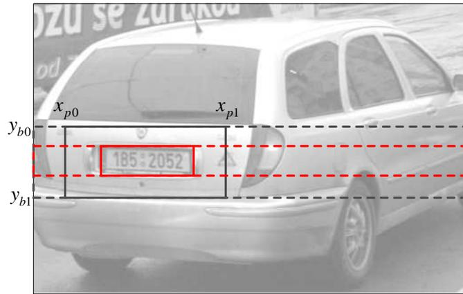
**Figure 2.4:** The double-phase plate clipping. Black color represents the first phase of plate clipping, and red color represents the second one. Bands are represented by dashed lines, and plates by solid lines.
