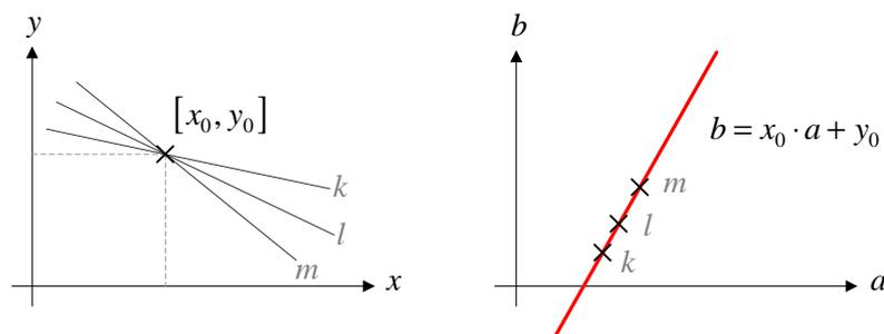
**Figure 2.11:** The “XY” and “AB” (“Hough space”) coordinate systems. Each point  $[x_0, y_0]$  in the “XY” coordinate system corresponds to one line in the Hough space (red color). There are several points (marked as  $k, l, m$ ) in the Hough space, that correspond to the lines in the “XY” coordinate system, which can cross the point  $[x_0, y_0]$ .
