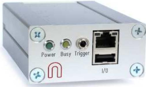
Figure 2.3: The SP1 stereo vision system.
