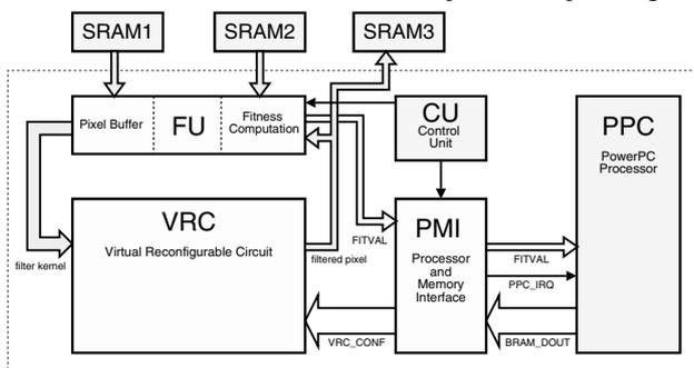
The CU is a hardwired controller which plays the role of master and controls the entire system. In particular, it starts/stops the evolution, determines the number of generations and other parameters of EA and generates the control signals for the remaining components. Considering the throughputs of buses and interfaces, this design alternative represents the most flexible and powerful solution.
