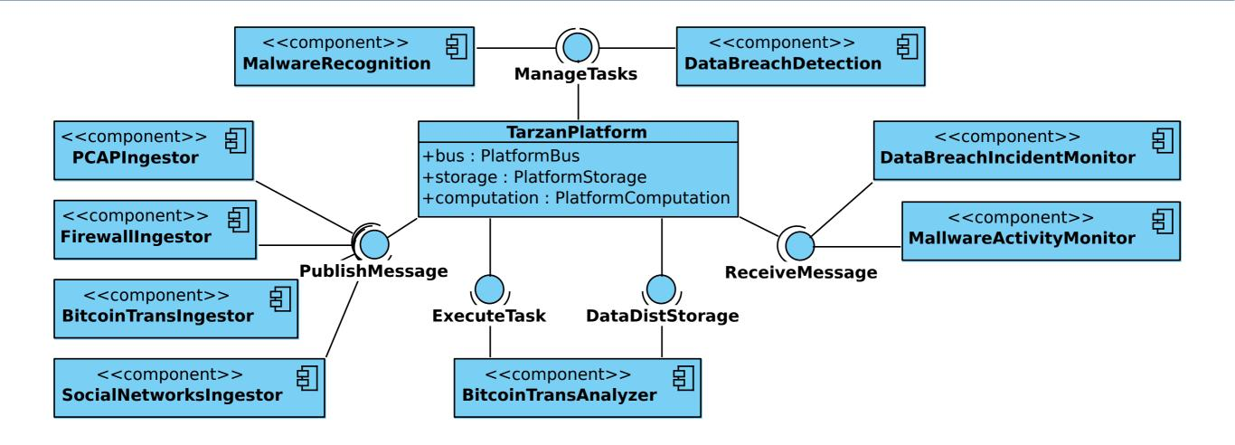
Fig. 3. An example of external application components utilizing the TARZAN Platform (the ingestors on the left side are feed data to the platform, computation tasks and an application on the top and bottom are processing the data, and the monitors on right side are passing results to clients).
