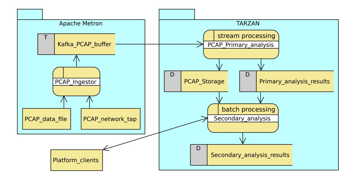
Fig. 4. Architecture of the PCAP Analysis tool with data-flows (including processes, data storages, and external data sources and entities).
