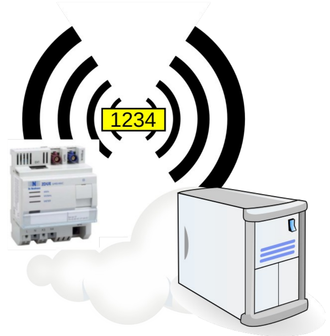
advanced metering infrastructure (AMI)
