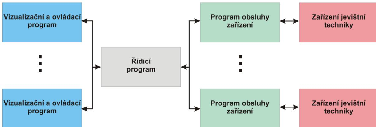
Fig. 1. Block diagram of a typical stage technology system
