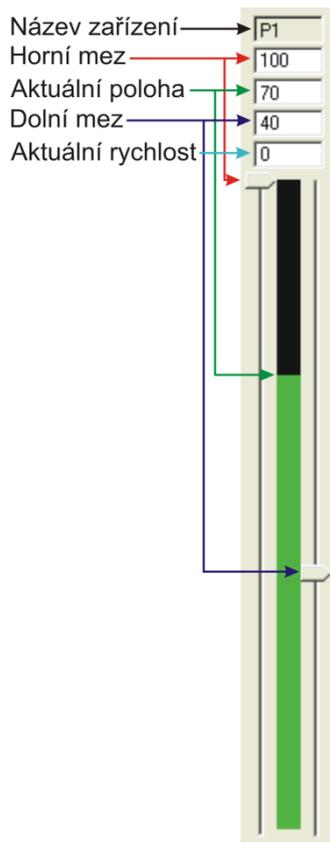
Fig. 5. The appearance of the device on control lever
