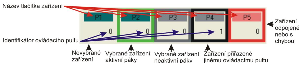
Fig. 4. Various forms of the device control buttons
