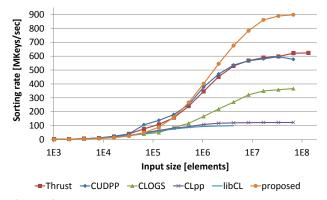
**Figure 4.** Sorting rates on 32-bit key-value pairs (higher is better).
