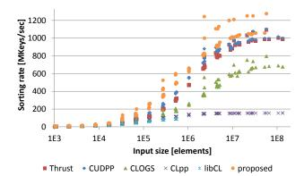
**Figure 5.** Sorting rates on 32-bit key-value pairs, keys were generated in sparse matrix multiplication (higher is better).
