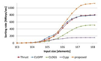
Figure 3. Sorting rates on 32-bit keys (higher is better).
