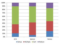
**Figure 1.** Relative amount of time spent in different phases of sparse matrix multiplication on GPU.
