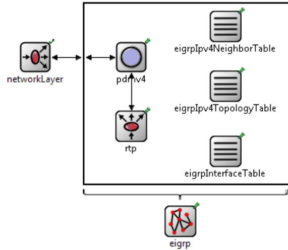
Figure 2: EIGRP simulation module structure
