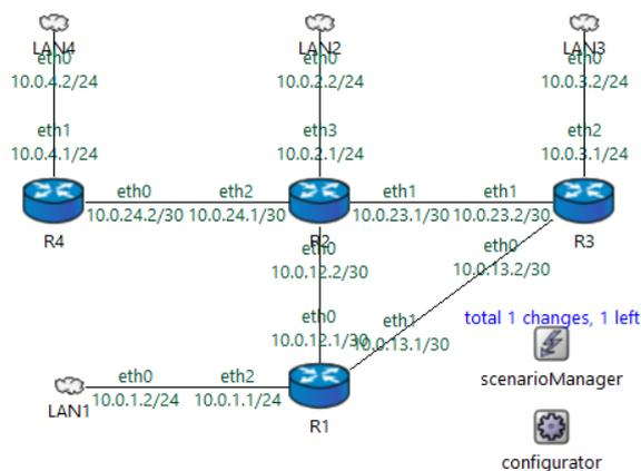
Figure 3: EIGRP testing topology
