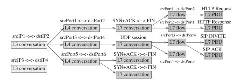
Fig. 2. Extraction of L7 PDUs from input packets.
