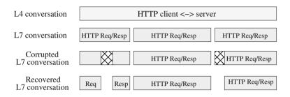
Fig. 3. Recovery of corrupted conversations.
