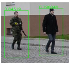
Figure 16: The gun of the soldier on the left hand side of the image was previously detected. The civilian has no gun.
