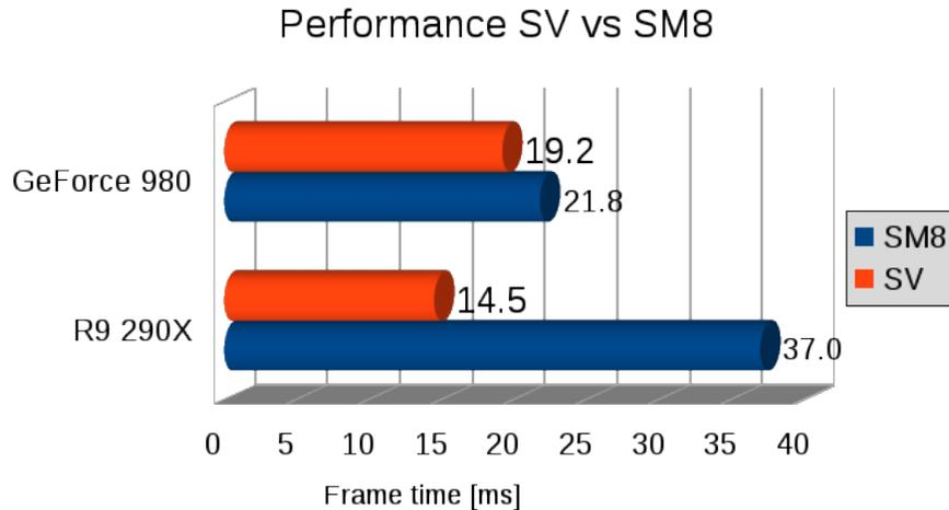
Graph 1: Performance comparison between our shadow volumes (SV) and standard omnidirectional shadow mapping with resolution 8192x8192x6
