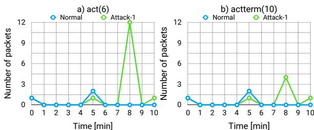
Figure 7: Distribution of (a) Act packets and (b) ActTerm packets during the normal usage and during the attack.
