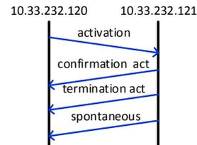
Figure 6: IEC 104 node activation command sequence
