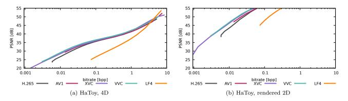
Fig. 4: Comparison of the image quality (PSNR/bitrate) computed between (a) original 4D bodies and (b) 2D views rendered from 4D LF for multiple focal planes (average for 10 focal planes).
