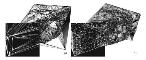
Fig. 3. Initial mesh (a) and result of the iterative adaptation (b).
