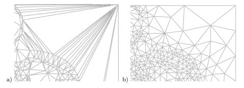
Fig. 2. 2D Delaunay triangulation constructed by the plain incremental method (a) and result of the isotropic meshing (b).
