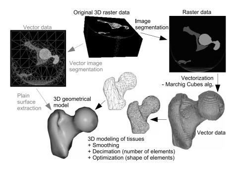
**Fig. 1.** Comparison of the traditional raster-based segmentation (black labeling) and the proposed vector segmentation method (underlined).
