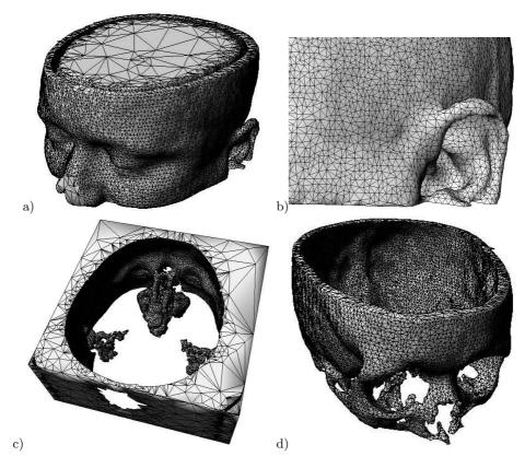
Fig. 4. Result of the vector segmentation. Polygonal surfaces of meaningful image segments extracted directly from the classified tetrahedral mesh: soft tissues (a,b), hard tissues (c), and bacground/air (d).
