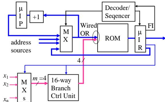
**Fig.5. Micro-programmed controller architecture with multi-way branching**
