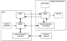
Testing environment is described as a composition of a tester and a set of external system simulators. Tester automatically executes specific test scripts and coordinates the SUT via a man machine interface (MMI) and the external system simulators. Set of external system simulators interact with SUT and simulate a tested environment (e.g. a behaviour of field objects as points, track circuits, coloured signals, etc.). Computer based control system (CBCS):
