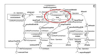
Component "testEnvironment" is able to receive component "test" (a test script) and to attach it as its sub-component via component "controller".
