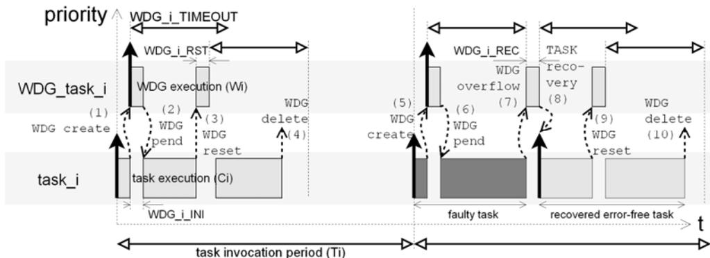
Fig. 4 – An Illustration to Timings Related to Error-Free and Faulty Tasks
