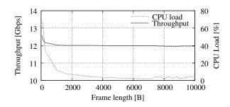
Figure 2: Achieved throughput and CPU utilization for various length of packets
