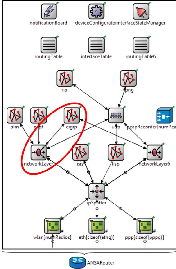
Figure 1: ANSARouter structure with highlighted contribution.
