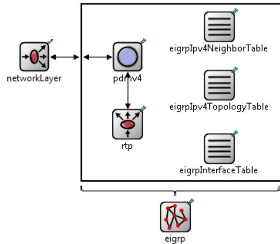
Figure 2: EIGRP simulation module structure
