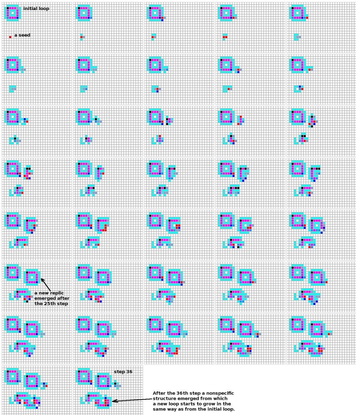
Figure 6: Part 1 of the replication according to the transition function from Figure 5. The sequence of steps reads from left to right and top to bottom. The development shows a replication of the initial loop (the upper part of each step) and a growth of a non-specific structure from a seed allowing to create the loop autonomously (the lower part of each step). The seed is represented by a cell in state 7.
