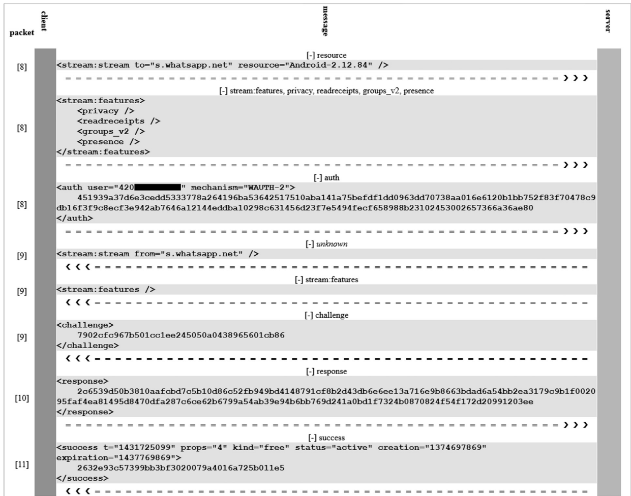
Fig. 1. Full handshake between WhatsApp client and server. Note: Numbers on the left side represent packet numbers (see Appendix A for the source pcap file). Also, there can be multiple messages in one packet.
