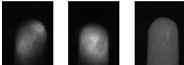
Figure 14.8 Fingertip illuminated using LED of 400 (left), 470 (middle) and 525 nm (right)
