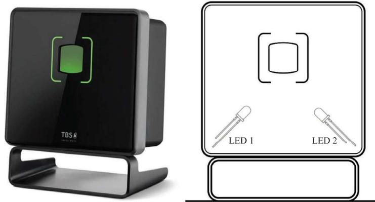
Figure 14.10 Fingerprint acquisition device [21] (left) and hardware modification for liveness detection (right)
