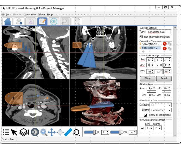
The predicted acoustic and thermal output is calculated using remote HPC resources managed by the dispatch server module. A successful treatment plan can be exported to an ultrasound therapy device for patient delivery.
