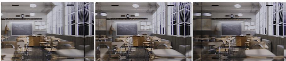
**Fig. 3** The *classroom* scene from the testing dataset was displayed on the LKG. Three photos were taken from different angles around the display showing the 3D parallax
