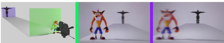
**Fig. 11** The first picture shows the 3D scene with two zero parallax plane positions. The second and third pictures are the actual results displayed on the LKG showing how the plane position affects the focusing in the rendered image
