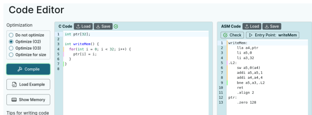
Fig. 4. Code editor displaying C and Assembly codes, with compiler parameters and control buttons.
