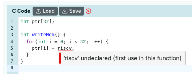
Fig. 6. Syntax error visualization in the C code.
