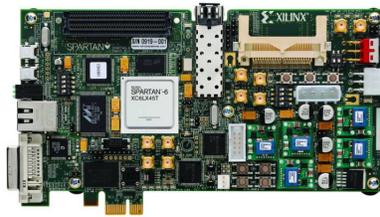
Figure 1: Spartan-6 SP605 FPGA kit.
