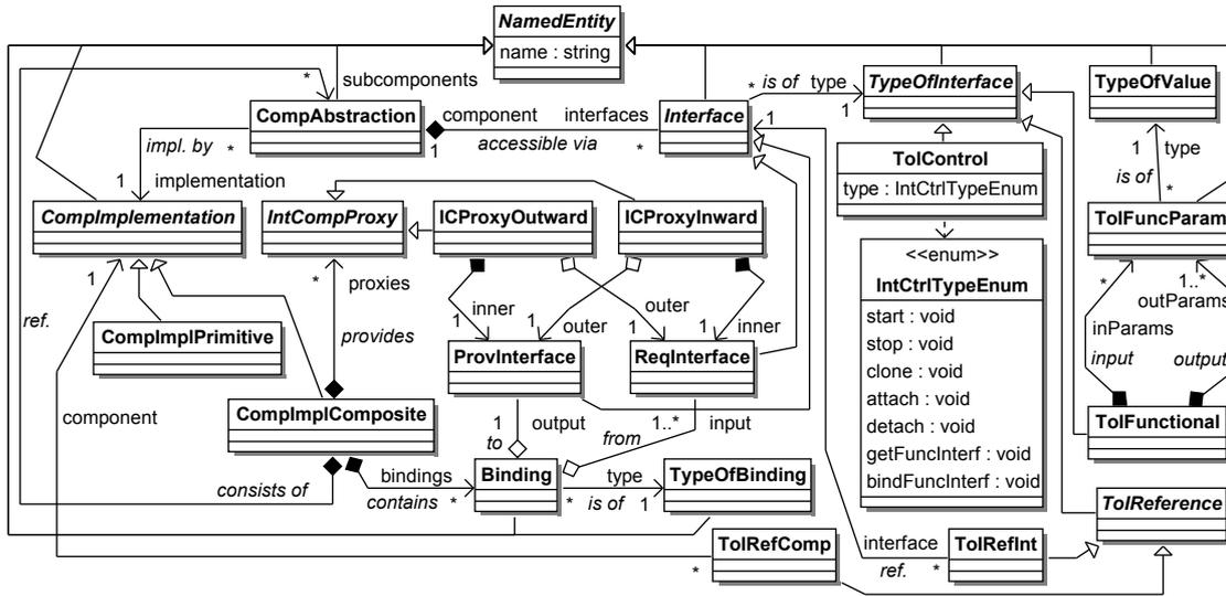
Figure 1: The meta-model of the component model (the UML notation [11]).
