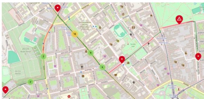
Fig. 5: Visualization of the computed route with traffic analysis from 1 Dec 2024 to 6 Jan 2025. Color-coded segments represent congestion levels, while traffic events are displayed as distinct icons. Events can also be grouped into clusters, with a numeric label indicating each cluster's total number of incidents.
