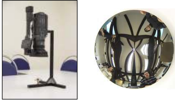
Figure 2: Omni-directional system and the hyperbolic mirror, as seen by the camera
