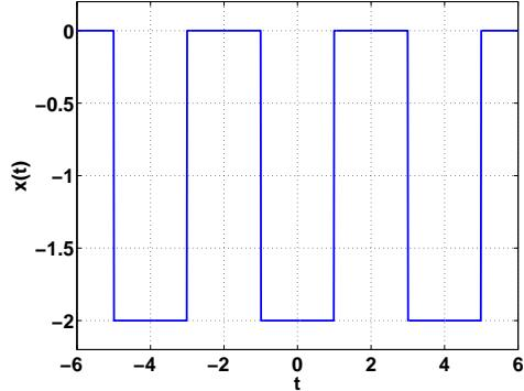
$$\begin{array}{c|c} \text{A} & \text{B} \\ c_k = \begin{cases} \text{sinc}(k\frac{\pi}{2})e^{-jk\frac{\pi}{2}} & \text{pro } k \neq 0 \\ 0 & \text{pro } k = 0 \end{cases} & c_k = \begin{cases} \text{sinc}(k\frac{\pi}{2})e^{+jk\frac{\pi}{2}} & \text{pro } k \neq 0 \\ 0 & \text{pro } k = 0 \end{cases} \\ \hline \text{C} & \text{D} \\ c_k = \text{sinc}(k\frac{\pi}{2})e^{+j\pi} & c_k = \text{sinc}(k\frac{\pi}{2})e^{+j\frac{\pi}{2}} \end{array}$$
