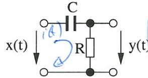
$$RC \frac{dx(t)}{dt} = y(t) + RC \frac{dy(t)}{dt}$$
