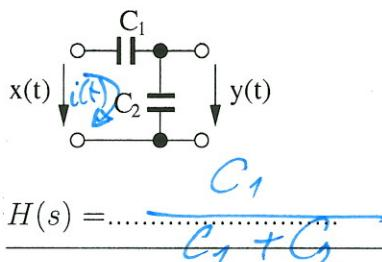
$$\begin{aligned} i(t) &= C_1 \frac{d(x(t) - y(t))}{dt} = C_1 \frac{dx(t)}{dt} - C_1 \frac{dy(t)}{dt} \\ i(t) &= C_2 \frac{dy(t)}{dt} \\ C_1 X(s)s - C_1 Y(s)s &= C_2 Y(s)s \quad C_1 X(s) = (C_1 + C_2)Y(s) \end{aligned}$$
