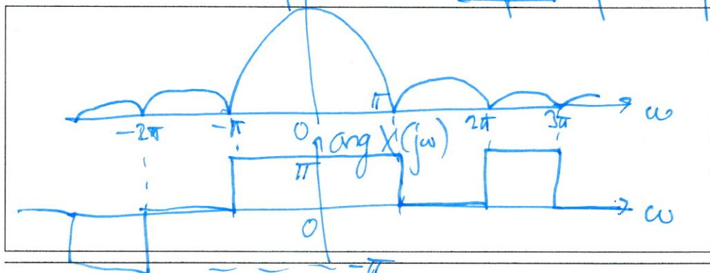
$$\begin{aligned} x(t) &= \begin{cases} -1 & -1 < t < 1 \\ 0 & \text{jinde} \end{cases} \\ X(j\omega) &= -D \text{sinc}\left(\frac{\omega}{2}\right) \\ &= -2 \cdot 2 \text{sinc}(1 \cdot \omega) \\ &\text{protíná osu } \omega \text{ pro } \pi. \end{aligned}$$
