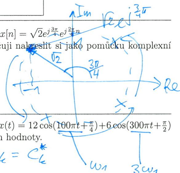
$$c_1 = 6e^{j\frac{\pi}{4}} \quad c_{-1} = 6e^{-j\frac{\pi}{4}} \quad c_3 = 3e^{j\frac{\pi}{2}} \quad c_{-3} = 3e^{-j\frac{\pi}{2}}$$
