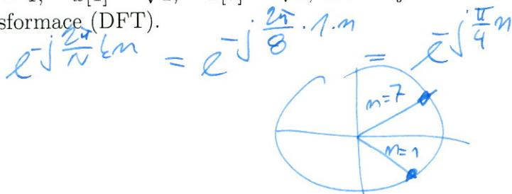
$$\begin{aligned} \text{pro } n=0 &\Rightarrow 1 \\ n=1 &\Rightarrow e^{-j\frac{\pi}{4}} = +\frac{1}{\sqrt{2}} - j\frac{1}{\sqrt{2}} \\ n=7 &\Rightarrow e^{-j\frac{7\pi}{4}} = +\frac{1}{\sqrt{2}} + j\frac{1}{\sqrt{2}} \end{aligned}$$
