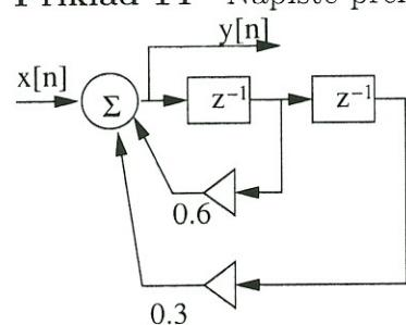
$$\begin{aligned} Y[n] &= x[n] + 0.6 Y[n-1] + 0.3 Y[n-2] \\ Y(z) &= X(z) + 0.6 Y(z) z^{-1} + 0.3 Y(z) z^{-2} \\ Y(z) (1 - 0.6 z^{-1} - 0.3 z^{-2}) &= X(z) \end{aligned}$$
