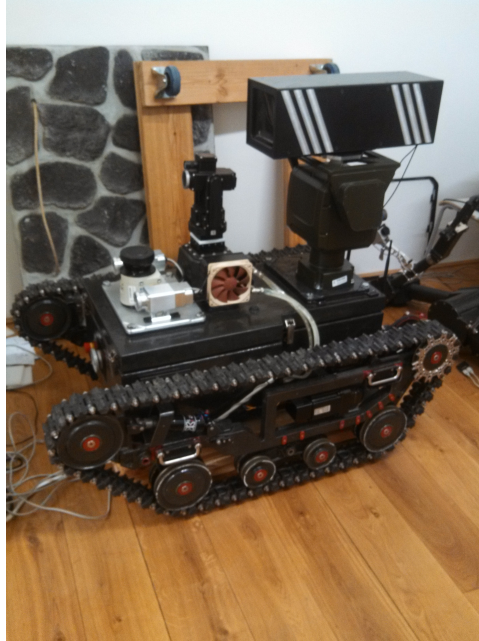
Figure 5.1: Sensoric system installed on experimental robot RUDA.
