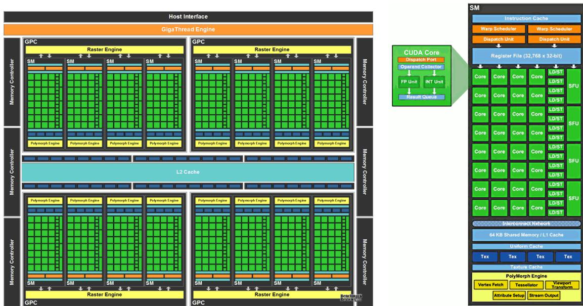
Figure 2.13: Fermi Architecture GeForce GT300 (GF100).
