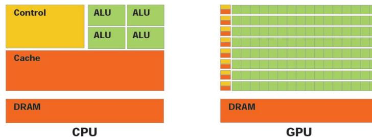
**Figure 2.5:** CPU and GPU Architecture Overview. [64]
