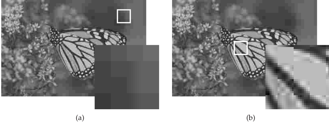
Figure 2.5: The JPEG artifacts in the form of the blocking (a) on the left and ringing (b) on the right which is visible on the edges. The monarch image is here compressed with the quality 10 and it is selected from LIVE1 image dataset [22].
