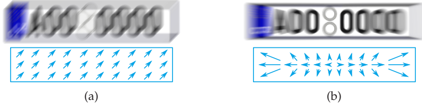
Figure 2.1: An uniform motion blur (a) with a vector field representing the spatial blur and a non-uniform blur (b).
