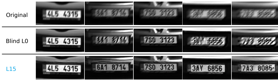
Figure 6.7: The naturally blurred license plates sorted from left to right based on the blur amount with the corresponding deconvolved results of L0-regularized method and the restored L15 images.
