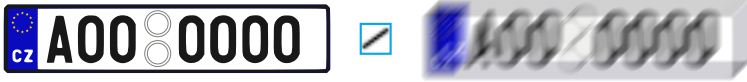
Figure 2.2: The sharp image x blurred with the motion blur PSF g . The result is an uniformly blurred image y .
