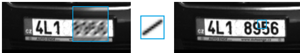
Figure 4.3: The training image pair with the illustrated blurred crop on the left and the equivalent sharp center patch on the right. In the middle is the magnified motion blur PSF.
