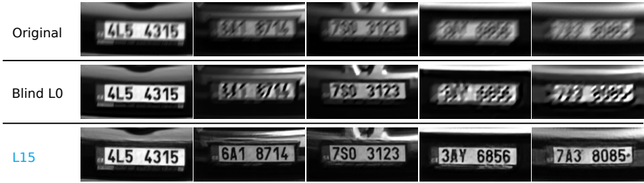
Figure 4.6: The naturally blurred license plates sorted from left to right based on the blur amount with the corresponding deconvolved results of L0-regularized method and the restored L15 images.
