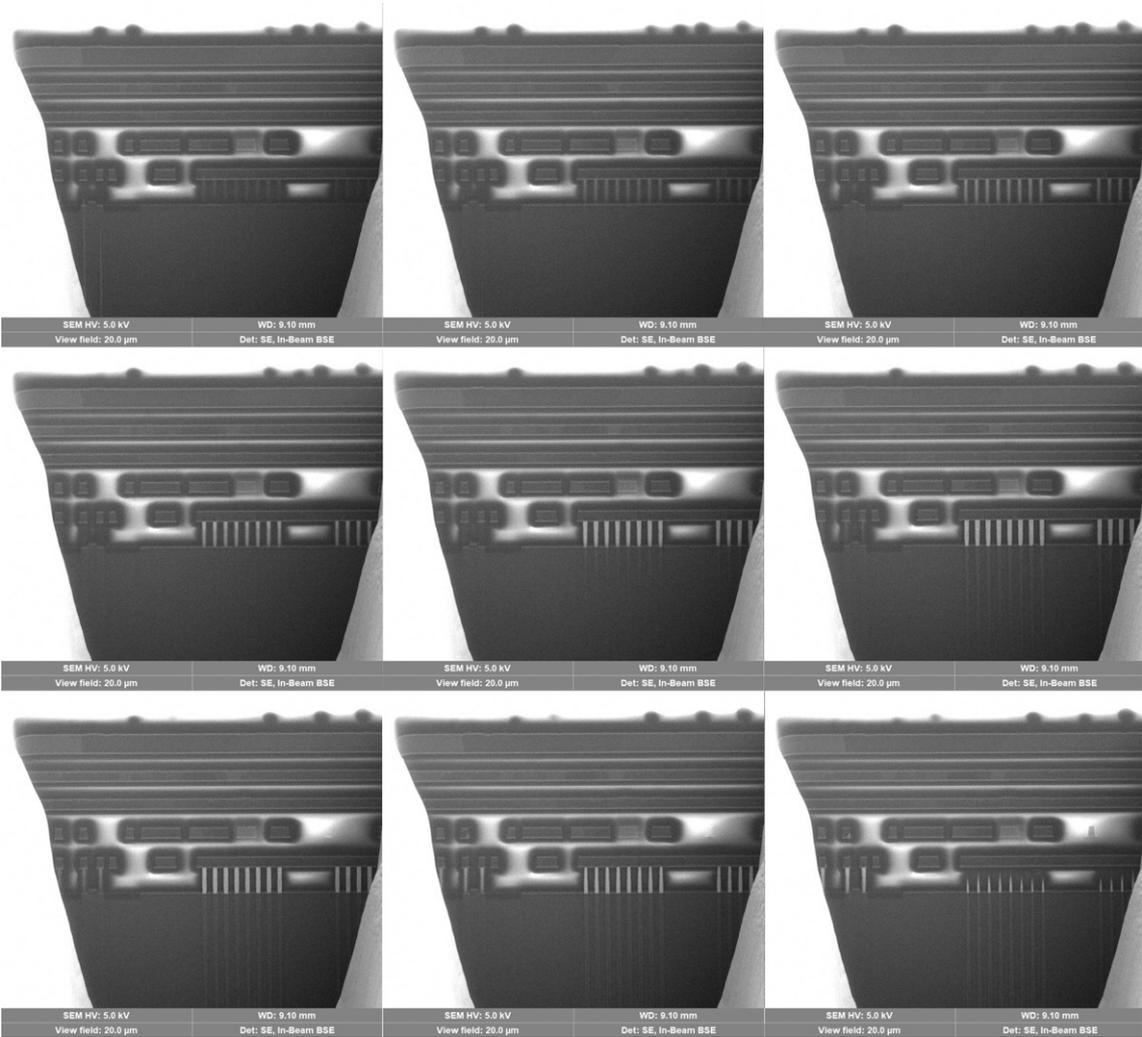
Figure A.1: FIB milling performed on the NXP P5CD080 V0B; cross-section images are scanned after 50 nm milling step. (Source: author's work.)
