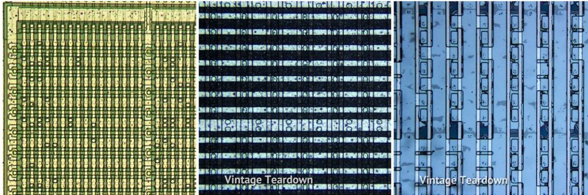
Figure 3.2: Various types of Mask ROM acquired by an optical microscope. (Sources: [119], [156])
