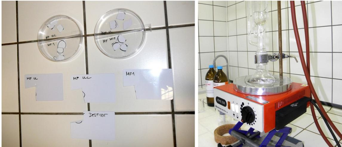
Figure 7.1: Initial phase of the microscopic analysis—obtaining the chips. Left: RFID chips in typical plastic cards. Right: Boiling nest with acetone bath. (Source: author’s work.)
