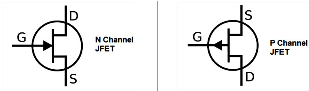
Figure 2.1: Unipolar JFET transistor schematic. Left: n-type; Right: p-type. (Source: [94])
