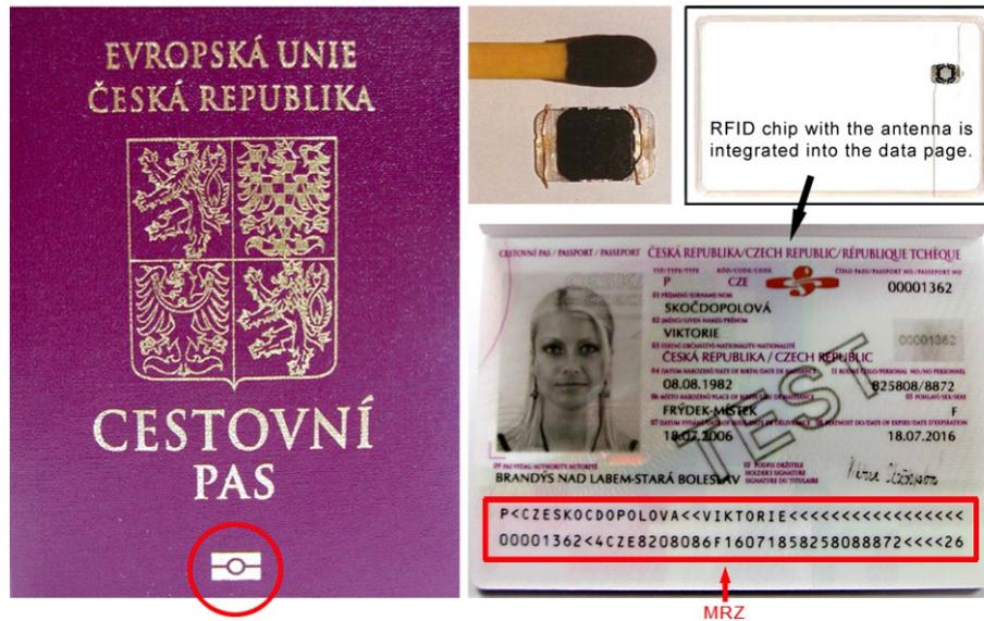
Figure 6.1: Left: A Czech biometric passport specimen with a circled international logo of electronic passports. Top right: RFID chip without and with an antenna. Bottom right: The data page with labeled MRZ. (Source: [64])
