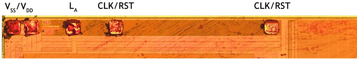
Figure 8.10: Bondpads in the top edge of chip NXP P5CD080 V0B. (Source: author's work.)
