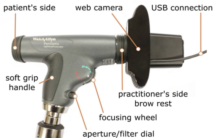
Fig. 3.3: Setup with Welch Allyn Panoptic Ophthalmoscope.
