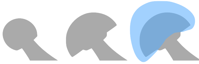
Figure 5.6: A femoral stem with attached ball head (left), ball head occluded by the acetabular prosthesis (middle), blue colored drop-out area roughly selected by a user (right).
