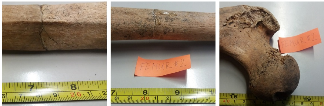
Figure 9.8: Transverse diaphyseal fractures of cadaveric bones ( left and middle ). Degraded greater trochanter of the second femur ( right ).
