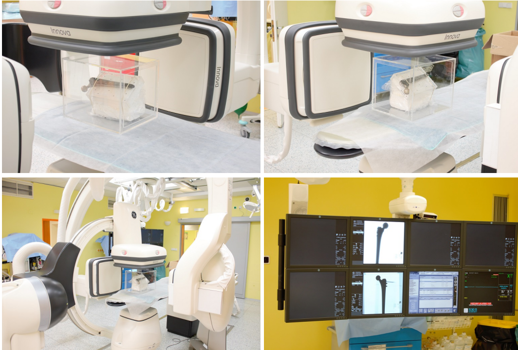
Figure 5.10: Capturing radiographs of femoral stem using Innova fluoroscope.
