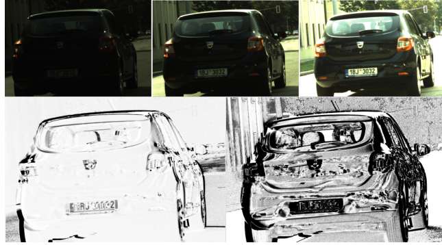
Figure 4.2: Two Certainty maps (bottom) obtained from the sequence on the top. The Certainty map on the left was obtained from top left and top middle (reference) image, the Certainty map on the right was obtained from top middle (reference) and top right image.
