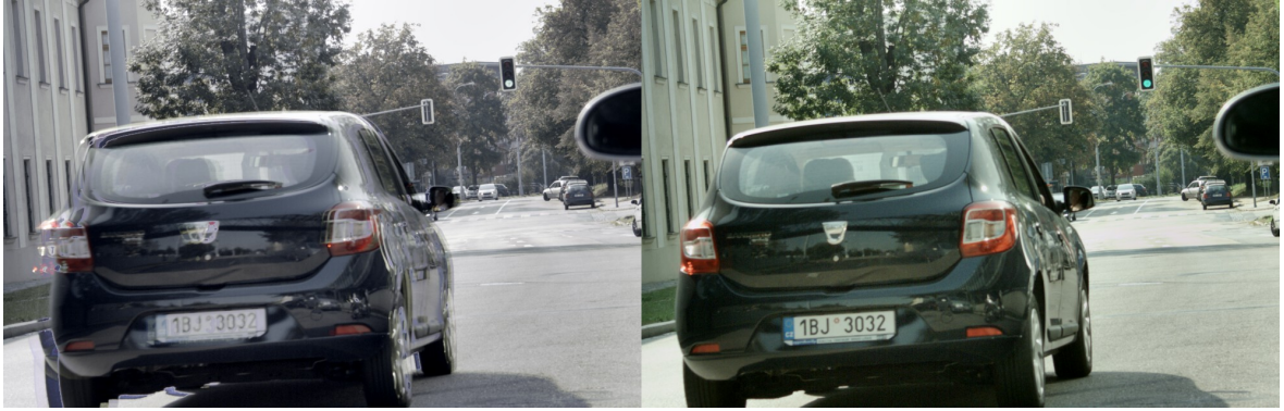
Figure 4.12: A car passing by the camera – ghosted HDR (left) and result of the proposed ghost-free merging algorithm (right).
