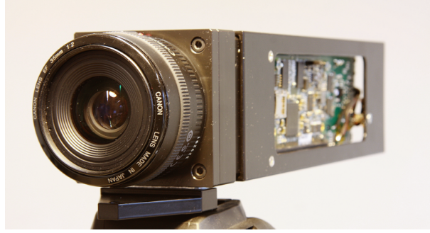
Figure 3.5: Prototype of HDR camera by Nosko et al. [30, 31]
