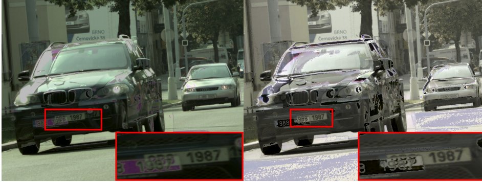
Figure 4.6: Sample outputs of related deghosting algorithms by Pece et al. [32] (left) and Min et al. [26] (right) on the scene from Figure 4.1. Our experiments revealed that listed algorithms should be successful only on images with convenient histogram distribution.
