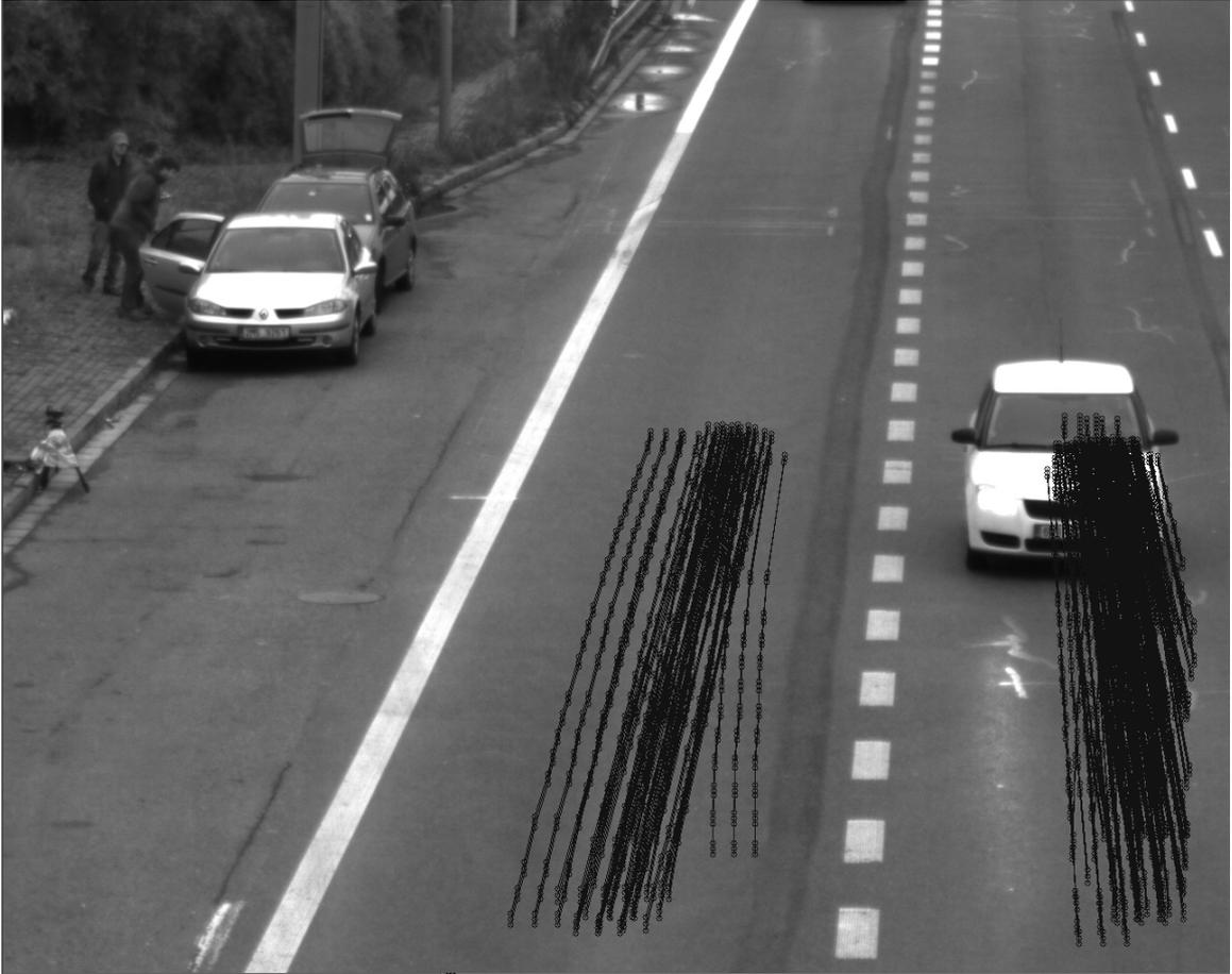
Figure 6.6: The area covered by the passes of the calibration vehicles through the measured road section is shown. Nine tracks that correspond to the extracted license plate points are drawn for each calibration vehicle.
