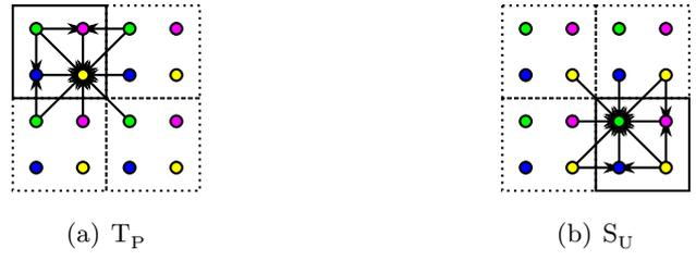
Figure 8.11: 2-D dataflow diagram, CDF 5/3 wavelet, Monolithic scheme. The solid box corresponds to the output coefficients.
