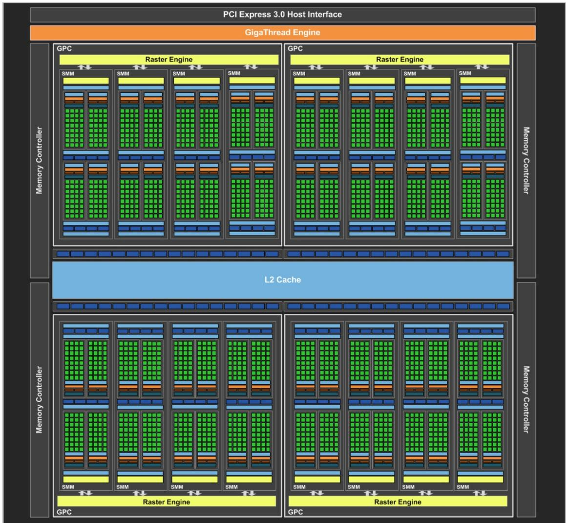
Figure 2.2: Block diagram of Maxwell GM204 GPU platform which can be found in Nvidia GeForce GTX 980 GPU. The GPU consists of: Main scheduler denoted as GigaThread Engine, four Memory Controllers located on the sides of block diagram each connected to a GDDR5 global memory chip by 64bit bus, 2MB of L2 cache for caching global memory load/store operations, and 16 Multiprocessors denoted as SMM (Streaming Maxwell Multiprocessor) grouped into 4 GPC (Graphics Processing Clusters) [3].
