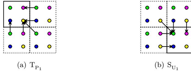
Figure 8.15: 2-D dataflow diagram, CDF 5/3 wavelet, Monolithic\* scheme. The solid box corresponds to the output coefficients.
