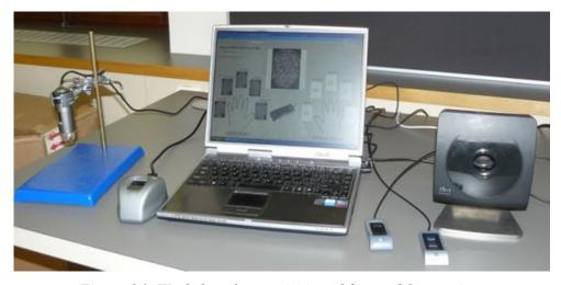
Figure 6.1: Workplace for acquisition of diseased fingerprints.
