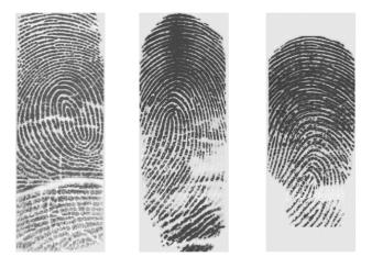
Figure 5.1: Examples of real fingerprints from swipe sensor.
