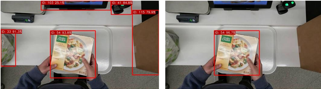
FIGURE 4.13: Detection of products without/with the usage of detected ROI.
