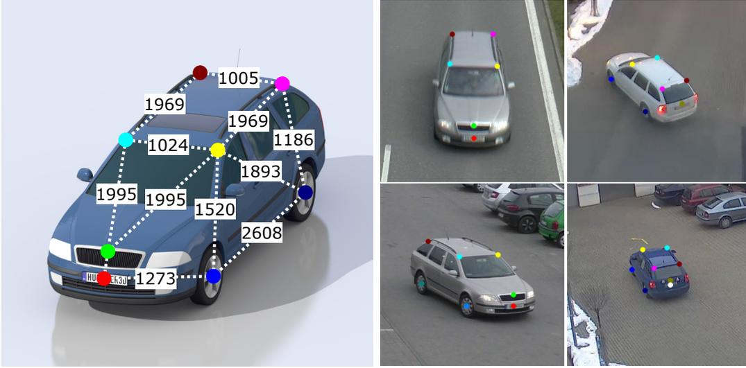
FIGURE 3.6: *left*: Distances  $\hat{\delta}$  (in millimeters) in the 3D model of *Skoda Octavia mk2* car. Only a small subset of all the distances in the set  $\hat{\mathcal{K}}^{c_i}$  is shown. *right*: Examples of detected landmarks on actual vehicles of the same type.
