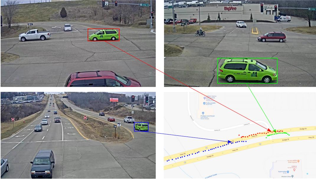
FIGURE 4.8: Example result of our positional matching method with a projection of trajectory points into a linear coordinate system. Arrows depict transformed points from image space to real-world space in a specific time-step (displayed camera frame).
