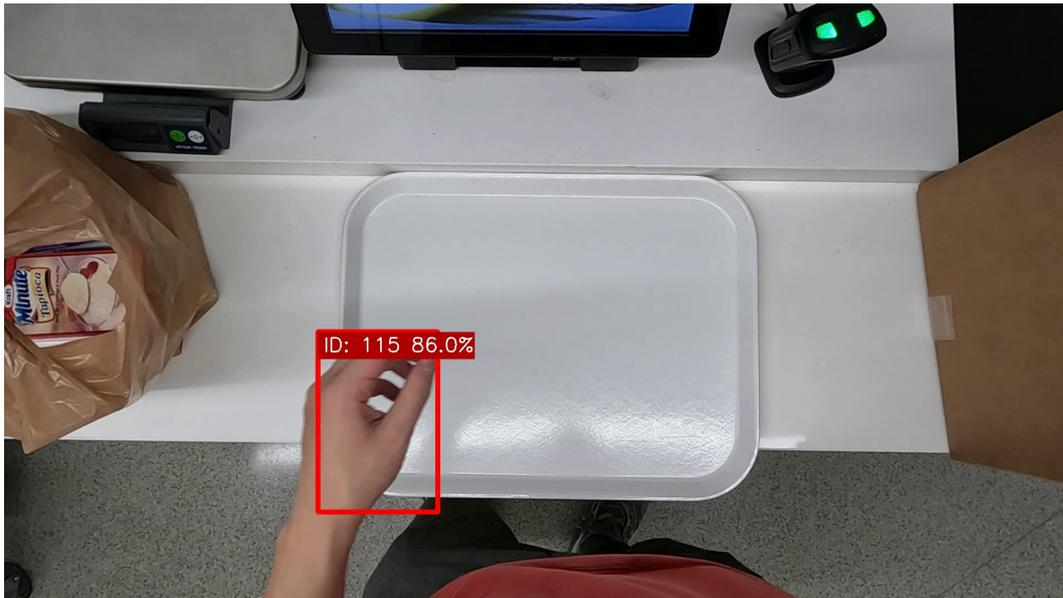
FIGURE 4.10: False positive product detection on person body in original frame.
