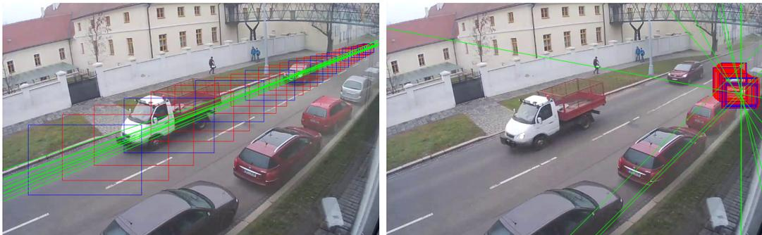
FIGURE 5.3: An example of computing the trajectory contribution value. Rectangles are observations, and endpoint observations of the trajectory parts are blue. Direction vectors  $\vec{v} = \mathbf{t}(b)^{\mathbf{P}} - \mathbf{t}(a)^{\mathbf{P}}$  for each consequent couple of endpoint indices  $a, b$  are shown as green lines. **left:** Typical movement in the single dominant direction (car on the road). **right:** Motion in an uncommon direction (car leaving parking place).
