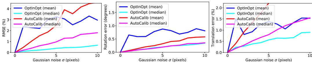
FIGURE 3.22: Calibration accuracy by the proposed method *OptInOpt* and by *AutoCalib* on synthetic dataset w.r.t. varying noise levels in 2D positions of landmarks. Random Gaussian shift with standard deviation  $\sigma$  is added to all 2D landmarks' positions. *left*: Calibration error, *center*: rotation error, *right*: translation error.
