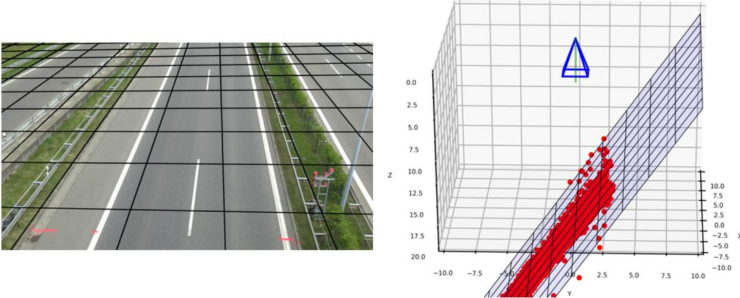
FIGURE 3.13: Final calibration plane with the use of all available cars in  $\mathcal{C}$ . *left*: 2D frame with the final calibration in WCS. *right*: 3D CCS with potential ground points and fitted plane.
