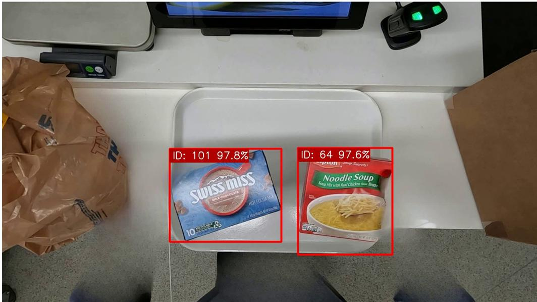
FIGURE 4.15: Multi-class detection with our trained *YOLOX* detector.
