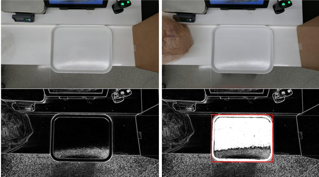
FIGURE 4.14: *Top row*: Mean background images for two sample scenes. *Bottom left*: Edges detection by the Scharr operator. *Bottom right*: Detection of the “tray” by the usage of flood fill algorithm; bounding rectangle in red.
