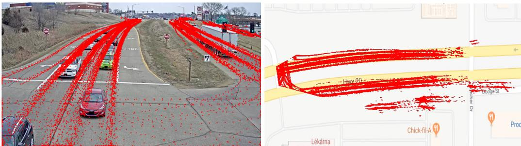
FIGURE 4.3: *left*: Detections' bottom points used for localization of camera's view area. *right*: Corresponding points transformed to the linear space (viewpoint selected as the convex hull of these points).
