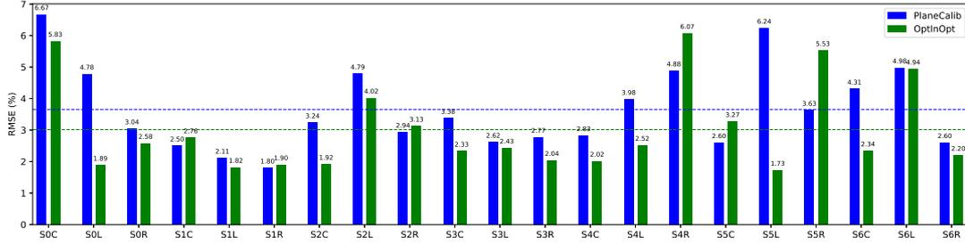
FIGURE 3.15: Comparison of accuracy for the proposed *PlaneCalib* method and the *OptInOpt* method. Average results are as follows: *PlaneCalib* 3.65%, *OptInOpt* 3.01%. These results are measured when calibrating from all the input samples; further, a mechanism for the selection of a more suitable subset is discussed.
