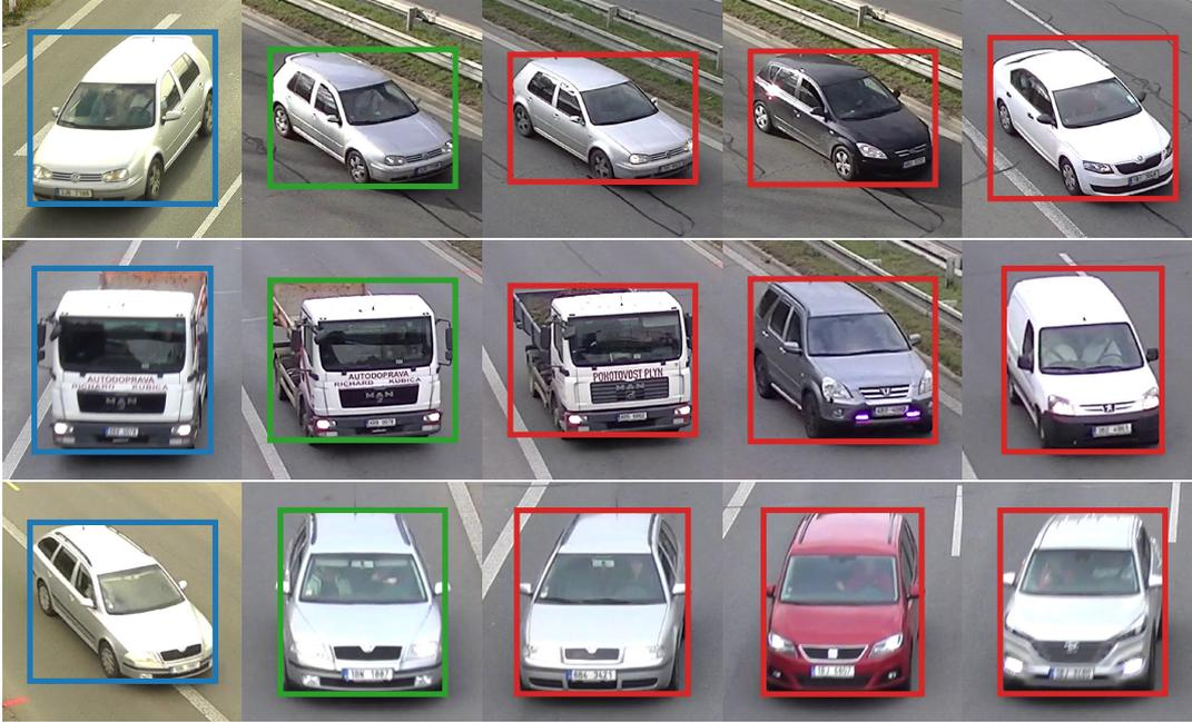
FIGURE 4.2: Examples of **queries**, **positive**, and **negative** samples. The negatives are sorted by difficulty from left to right (hard to easy) based on distances obtained from our re-identification feature vectors. It should be noted that the hardest negative sample has usually subtle differences (*e.g.* missing a small spoiler in the first row). Image source: [5].
