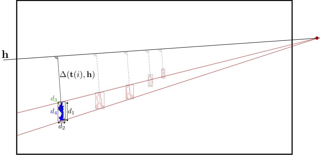
FIGURE 5.1: One possible trajectory (a few selected observations) in the video frame. Each observation consists of position  $\mathbf{t}(i)^{\mathcal{P}}$  and possible dimensions  $\mathbf{t}(i)^{\mathcal{d}}$ . The distance  $\Delta(\mathbf{t}(i), \mathbf{h})$  from horizon  $\mathbf{h}$  is also depicted.
