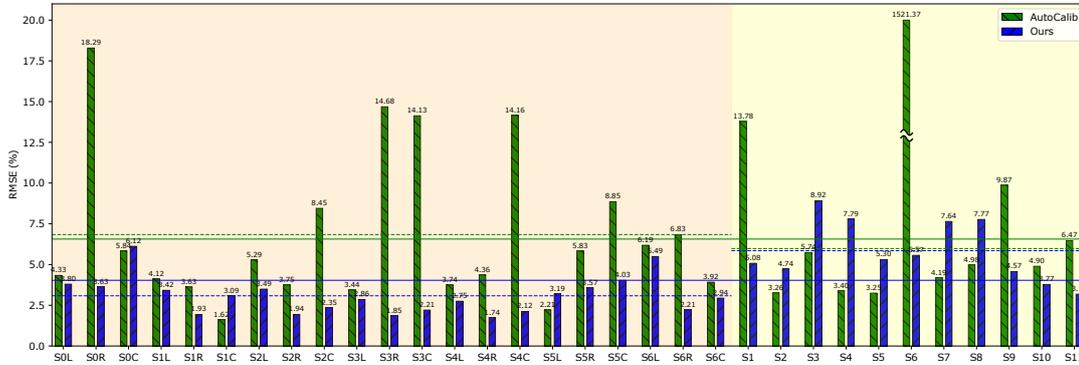
FIGURE 3.8: Comparison of accuracy for the proposed *LandmarksCalib* and *AutoCalib* method. Average results are as follows: *BrnoCompSpeed* dataset – *AutoCalib* 6.84 %, ours 3.08 %; *BrnoCarPark* dataset – *AutoCalib* 5.98 %, ours 5.84 % (it should be mentioned that *AutoCalib* failed significantly on scene *S6* and thus this single scene is not evaluated for *AutoCalib* method); both datasets — *AutoCalib* 6.56 %, ours 4.03 %.
