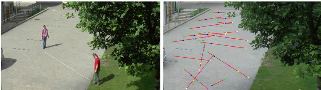
FIGURE 6.1: Experiments with more precise ground truth calibration measurements. *left*: Two people place a rope with regular marks (five 1 m sections in this case) into multiple locations in front of the camera. *right*: In a short and uncomplicated process, a high number of precise measurements can be obtained — for each rope placement, one frame of the video gives several very accurate distance measurements in the ground plane by manual or automatic recognition of the distance marks.
