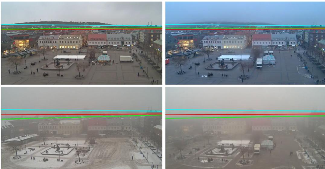
FIGURE 5.13: Resulting detected horizons for different recordings of the same scene (different lighting conditions, daytime, present objects, ...); *red*: ‘geometric’ horizon, *green*: horizon computed from the video, *cyan*: mean of human inputs
