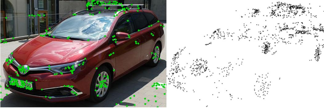
FIGURE 6.2: SfM reconstruction of a particular vehicle model, later used for accurate landmark localization. *left*: one frame of the source video, with the keypoints marked by green, *right*: reconstructed point cloud; points are candidate landmarks for the calibration.
