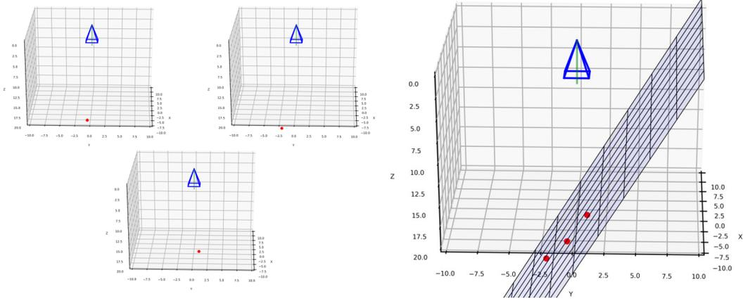
FIGURE 3.12: Computing the plane in the camera coordinate system. *left*: Origins of three different objects transformed into the camera coordinate system. *right*: plane in the camera coordinate system localized by three (minimal case) origins of objects.
