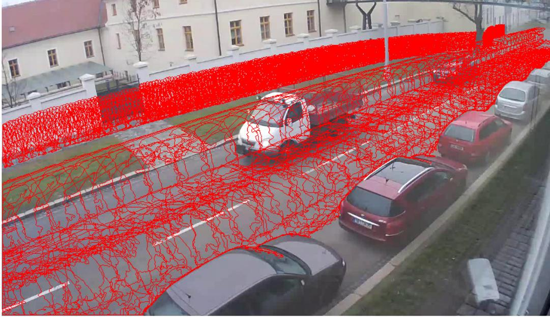
FIGURE 5.2: Example of a scene with one dominant direction of objects' motion. There are two directions of car movement on the road and a bidirectional stream of pedestrians on the sidewalk. Most of the tracks only testify to one vanishing point; only rare pedestrians crossing the road bring the missing information.
