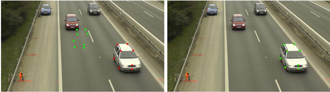
FIGURE 3.19: *left*: Projected 3D landmarks' positions  $\hat{\mathcal{K}}^{c_i}$  to the image plane (green points) and localized landmarks positions  $\tilde{\mathcal{K}}^{c_i}$  (red points). *right*: Projected 3D landmarks' positions  $\hat{\mathcal{K}}^{c_i}(\omega_\phi)$  (green points) after optimization of transformation parameters  $\omega_\phi$  and localized landmarks positions  $\tilde{\mathcal{K}}^{c_i}$  (red points).
