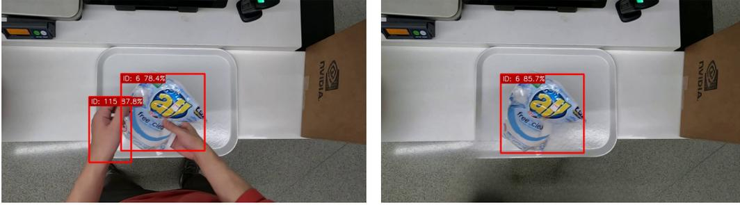
FIGURE 4.12: The difference between detection in the original and the inpainted frame.
