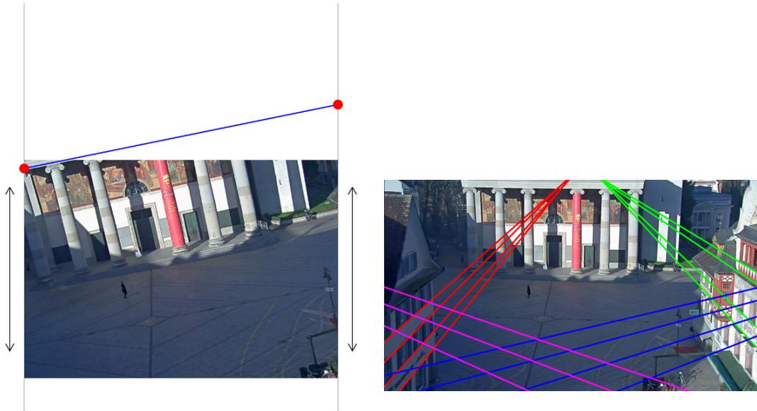
FIGURE 5.8: Scene horizon annotation principles. **left:** Web annotation tool for crowdsourced data collection. **right:** ‘Geometric’ ground truth annotation by using scene parallel lines.
