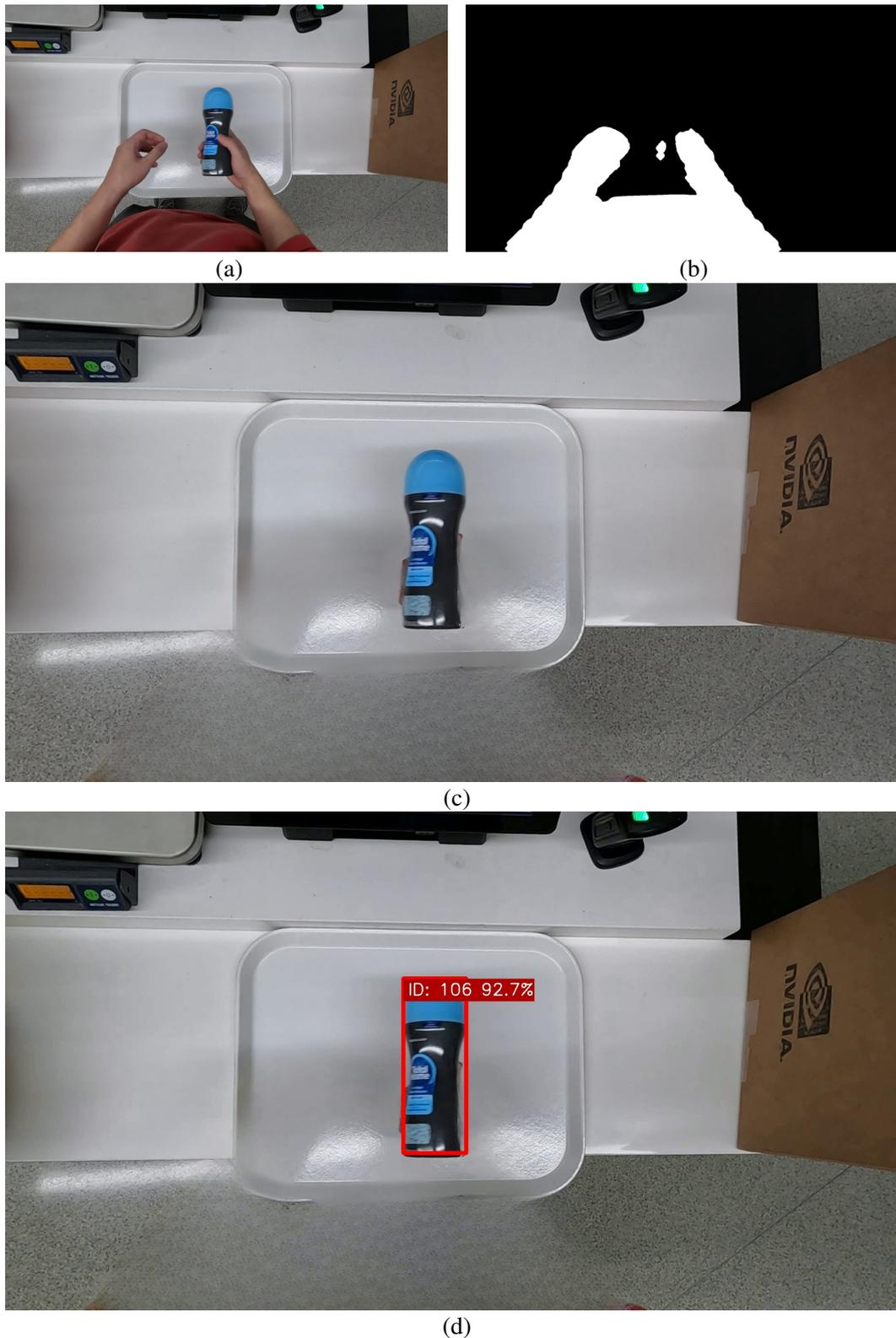
FIGURE 4.9: Our proposed solution for product detection. (a): Original video frame. (b): Detected mask of a person by CNN. (c): Removed “unwanted” parts by image inpainting algorithm. (d): Resulting detection of a product by CNN detector.
