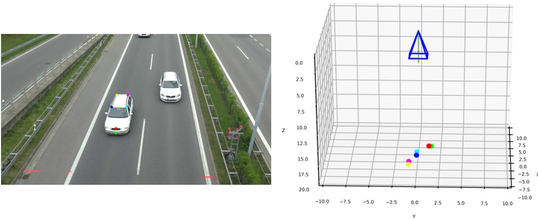
FIGURE 3.11: *left*: Detected 2D landmarks in a single frame. *right*: 3D CCS with corresponding 3D positions of detected landmarks in the 2D frame. The *PnP* solution is computed to obtain parameters  $[\mathbf{R}^{c_i} | \mathbf{t}^{c_i}]$ .
