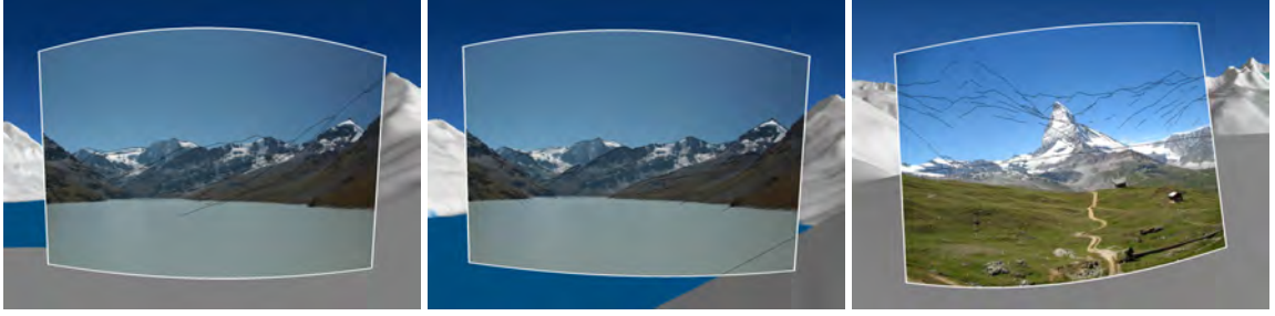
Figure 4.2: Example of a viable , but contaminated camera pose (left), refined camera pose (middle) and incorrect camera pose (right). Synthetic mountain silhouettes are overlaid with the aligned image. Image credit: left and middle image—Flickr.com user Michael Holtrop : https://www.flickr.com/photos/bartje_assen/2851555201/ , right image—Flickr.com user Bossi : https://www.flickr.com/photos/thisisbossi/2973222425/
