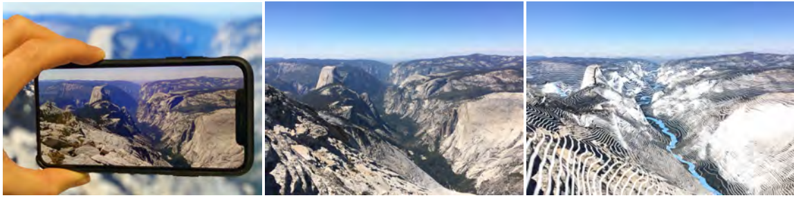
Figure 7.12: An iPhone application (in the left) is used to capture the photograph (in the middle) for which precise camera pose is estimated using our method. The estimated camera pose (in the right) is used to augment the query photograph with contour lines (white) and rivers (blue).
