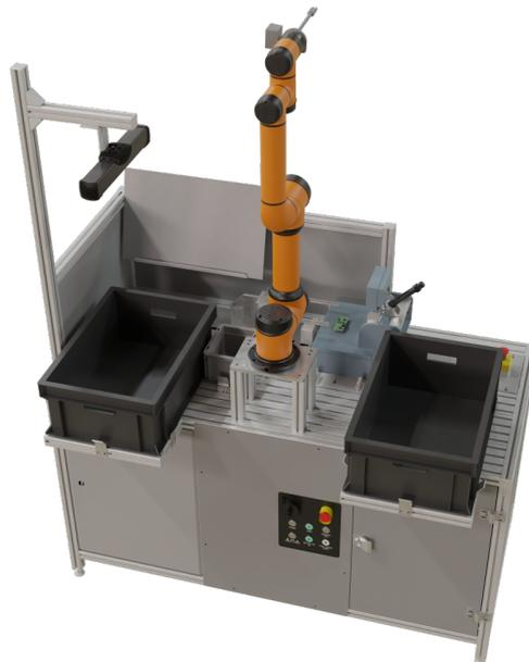
Figure 10.5: Render of a PCB testing workplace with the Ensenso 3D camera for bin-picking, 6 DoF AUBO i5 robot, 2 DoF custom-build robot, functional tester, barcode reader, and printer, source, and target boxes.
