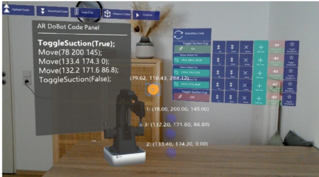
Figure 10.3: Robot Code, Robot Model in an AR application and block-based DSL Code (f.l.t.r.). Reprint from [62].
