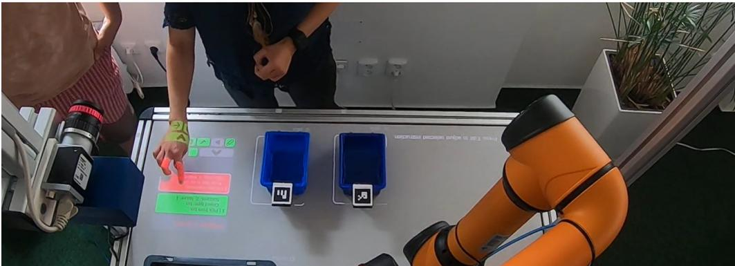
Figure 6.1: Participant programs a visual inspection task using the ARCOR SAR interface.
