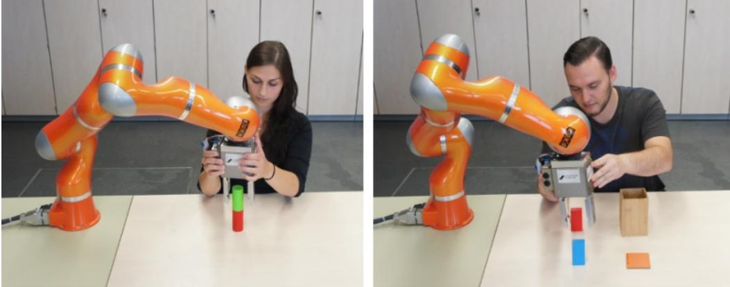
Figure 5.2: User programming the lightweight robot to solve a stacking (left) and sorting scenario (right). Reprint from [101].
