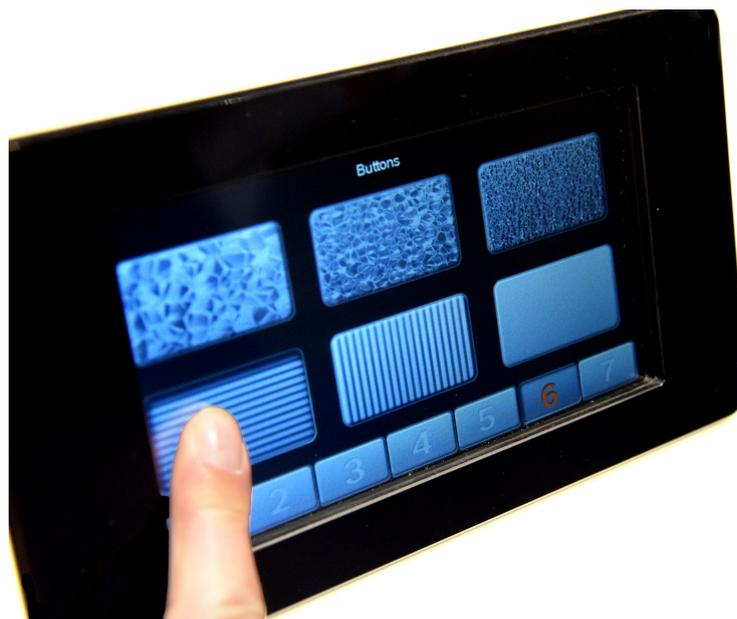
Figure 11.1: The touch screen device is equipped with a haptic feedback<sup>1</sup>. The 2D buttons provide feedback to the user, who can feel the button's texture with the tip of his finger.
