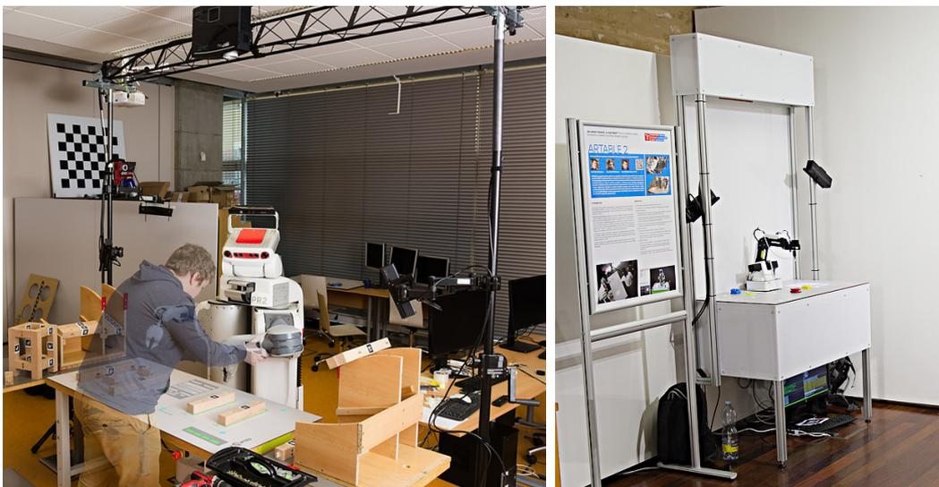
(a) The first generation of interactive table with projected SAR interface. (b) The second generation of interactive table with projected SAR interface.
