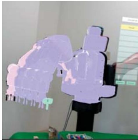
(b) After creating the waypoints, users can visualize the robot arm motion that is planned through the waypoints.
